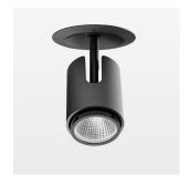
Semi-recessed luminaire with LED, rated life of the LED L80/B10 > 50000 h, chromaticity tolerance 3 SDCM (initial), , reflector with circular light distribution pattern, reflector pure aluminium 99,99% in MIRO-Silver®, segmented and faceted, exchangeable reflector unit in high-sheen black plastic, with glass cover, luminaire head die-cast aluminium, powder-coated, rotation angle 330°, swivel angle +90°/-90°, luminaire housing die-cast aluminium, powder-coated, stratoblack, separate driver unit
