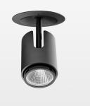
Semi-recessed luminaire with LED, rated life of the LED L80/B10 > 50000 h, chromaticity tolerance 3 SDCM (initial), , reflector with circular light distribution pattern, reflector pure aluminium 99,99% in MIRO-Silver®, segmented and faceted, exchangeable reflector unit in high-sheen black plastic, with glass cover, luminaire head die-cast aluminium, powder-coated, rotation angle 330°, swivel angle +90°/-90°, luminaire housing die-cast aluminium, powder-coated, stratoblack, separate driver unit
