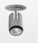
Semi-recessed luminaire with LED, rated life of the LED L80/B10 > 50000 h, chromaticity tolerance 3 SDCM (initial), , reflector with circular light distribution pattern, reflector pure aluminium 99,99% in MIRO-Silver®, segmented and faceted, exchangeable reflector unit in high-sheen black plastic, with glass cover, luminaire head die-cast aluminium, powder-coated, rotation angle 330°, swivel angle +90°/-90°, luminaire housing die-cast aluminium, powder-coated, stratosilver, separate driver unit
