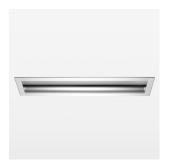
recessed luminaire with LED, rated life of the LED L80/B10 > 50000 h, color rendering index CRI > 90, chromaticity point tolerance 3 SDCM (initial), Reflector with asymerical light distribution pattern, 99.99% pure aluminium reflector made of MIRO-SILVER®, aluminium luminaire housing and frame, anodized, separate driver unit.
