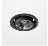
Recessed luminaire with LED, rated life of the LED L80/B10 > 50000h, colour rendering index CRI > 80, chromaticity tolerance 2 SDCM (initial), reflector with circular light distribution pattern, 99,99% pure aluminium, segmented and faceted, infinitely adjustable sheet steel luminaire housing, incl. glass cover, sheet metal powder coated, separate driver unit
