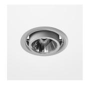
Recessed luminaire with LED, rated life of the LED L80/B10 > 50000h, colour rendering index CRI > 90, chromaticity tolerance 2 SDCM (initial), reflector with circular light distribution pattern, 99,99% pure aluminium, segmented and faceted, infinitely adjustable sheet steel luminaire housing, incl. glass cover, sheet metal powder coated, separate driver unit
