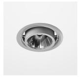
Recessed luminaire with LED, rated life of the LED L80/B10 > 50000h, colour rendering index CRI > 80, chromaticity tolerance 2 SDCM (initial), axially symmetrical reflector with circular light distribution pattern, 99,99% pure aluminium, segmented and faceted, infinitely adjustable sheet steel luminaire housing, incl. glass cover, sheet metal powder coated, separate driver unit
