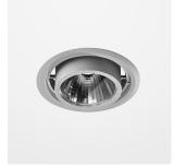
Recessed luminaire with LED, rated life of the LED L80/B10 > 50000h, colour rendering index CRI > 90, chromaticity tolerance 2 SDCM (initial), axially symmetrical reflector with circular light distribution pattern, 99,99% pure aluminium, segmented and faceted, infinitely adjustable sheet steel luminaire housing, incl. glass cover, sheet metal powder coated, separate driver unit
