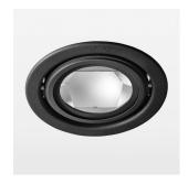
Recessed luminaire with LED, rated life of the LED L80/B10 > 50000 h, colour rendering index CRI > 90, chromaticity tolerance 2 SDCM (initial), reflector with circular light distribution pattern, reflector pure aluminium 99,99% in MIRO-Silver®, swivel angle +25°/-25°, luminaire housing sheet steel, powder-coated, stratoblack, separate driver unit
