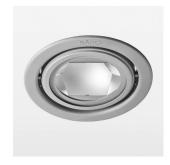
Recessed luminaire with LED, rated life of the LED L80/B10 > 50000 h, chromaticity tolerance 2 SDCM (initial), reflector with circular light distribution pattern, reflector pure aluminium 99,99% in MIRO-Silver®, swivel angle +25°/-25°, luminaire housing sheet steel, powder-coated, stratosilver, separate driver unit
