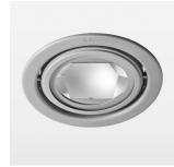
Recessed luminaire with LED, rated life of the LED L80/B10 > 50000 h, colour rendering index CRI > 90, chromaticity tolerance 2 SDCM (initial), reflector with circular light distribution pattern, reflector pure aluminium 99,99% in MIRO-Silver®, swivel angle +25°/-25°, luminaire housing sheet steel, powder-coated, stratosilver, separate driver unit
