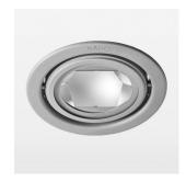
Recessed luminaire with LED, rated life of the LED L80/B10 > 50000 h, chromaticity tolerance 3 SDCM (initial), reflector with circular light distribution pattern, reflector pure aluminium 99,99% in MIRO-Silver®, swivel angle +25°/-25°, luminaire housing sheet steel, powder-coated, stratosilver, separate driver unit
