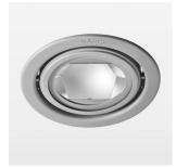
Recessed luminaire with LED, rated life of the LED L70/B10 > 50000 h, chromaticity tolerance 3 SDCM (initial), reflector with circular light distribution pattern, reflector pure aluminium 99,99% in MIRO-Silver®, swivel angle +25°/-25°, luminaire housing sheet steel, powder-coated, stratosilver, separate driver unit
