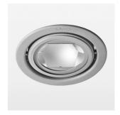
Recessed luminaire with LED, rated life of the LED L80/B10 > 50000 h, chromaticity tolerance 2 SDCM (initial), reflector with circular light distribution pattern, reflector pure aluminium 99,99% in MIRO-Silver®, luminaire head die-cast aluminium, powder-coated, swivel angle +25°/-25°, luminaire housing sheet steel, powder-coated, stratosilver, separate driver unit
