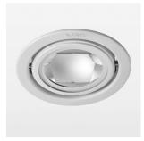
Recessed luminaire with LED, rated life of the LED L80/B10 > 50000 h, colour rendering index CRI > 80, chromaticity tolerance 3 SDCM (initial), reflector with circular light distribution pattern, reflector pure aluminium 99,99% in MIRO-Silver®, swivel angle +25°/-25°, luminaire housing sheet steel, powdercoated, stratowhite, separate driver unit
