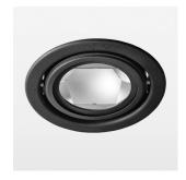
Recessed luminaire with LED, rated life of the LED L80/B10 > 50000 h, colour rendering index CRI > 80, chromaticity tolerance 3 SDCM (initial), reflector with oval light distribution pattern, reflector pure aluminium 99,99% in MIRO-Silver®, swivel angle +25°/-25°, luminaire housing sheet steel, powder-coated, stratoblack, separate driver unit
