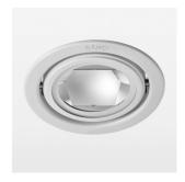
Recessed luminaire with LED, rated life of the LED L80/B10 > 50000 h, colour rendering index CRI > 90, chromaticity tolerance 2 SDCM (initial), reflector with oval light distribution pattern, reflector pure aluminium 99,99% in MIRO-Silver®, swivel angle +25°/-25°, luminaire housing sheet steel, powdercoated, stratowhite, separate driver unit
