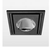
Recessed luminaire with LED, rated life of the LED L80/B10 > 50000 h, chromaticity tolerance 2 SDCM (initial), reflector with circular light distribution pattern, reflector pure aluminium 99,99% in MIRO-Silver®, swivel angle 30°, luminaire housing sheet steel, powder-coated, stratoblack, separate driver unit
