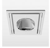
Recessed luminaire with LED, rated life of the LED L80/B10 > 50000 h, chromaticity tolerance 2 SDCM (initial), reflector with circular light distribution pattern, reflector pure aluminium 99,99% in MIRO-Silver®, swivel angle 30°, luminaire housing sheet steel, powder-coated, stratowhite, separate driver unit
