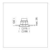
Recessed luminaire with LED, rated life of the LED L80/B10 > 50000 h, chromaticity tolerance 3 SDCM (initial), reflector with circular light distribution pattern, reflector pure aluminium 99,99% in MIRO-Silver®, swivel angle 30°, luminaire housing sheet steel, powder-coated, stratoblack, separate driver unit
