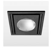
Recessed luminaire with LED, rated life of the LED L80/B10 > 50000 h, chromaticity tolerance 2 SDCM (initial), reflector with oval light distribution pattern, reflector pure aluminium 99,99% in MIRO-Silver®, swivel angle 30°, luminaire housing sheet steel, powder-coated, stratoblack, separate driver unit
