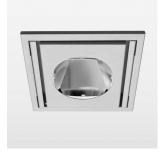
Recessed luminaire with LED, rated life of the LED L80/B10 > 50000 h, chromaticity tolerance 2 SDCM (initial), reflector with circular light distribution pattern, reflector pure aluminium 99,99% in MIRO-Silver®, swivel angle 30°, luminaire housing sheet steel, powder-coated, stratosilver, separate driver unit
