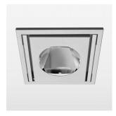
Recessed luminaire with LED, rated life of the LED L80/B10 > 50000 h, chromaticity tolerance 2 SDCM (initial), reflector with circular light distribution pattern, reflector pure aluminium 99,99% in MIRO-Silver®, swivel angle 30°, luminaire housing sheet steel, powder-coated, stratosilver, separate driver unit
