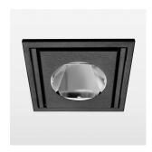
Recessed luminaire with LED, rated life of the LED L80/B10 > 50000 h, colour rendering index CRI > 90, chromaticity tolerance 2 SDCM (initial), reflector with circular light distribution pattern, reflector pure aluminium 99,99% in MIRO-Silver®, swivel angle 30°, luminaire housing sheet steel, powder-coated, stratoblack, separate driver unit
