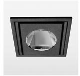
Recessed luminaire with LED, rated life of the LED L80/B10 > 50000 h, colour rendering index CRI > 90, chromaticity tolerance 2 SDCM (initial), reflector with circular light distribution pattern, reflector pure aluminium 99,99% in MIRO-Silver®, swivel angle 30°, luminaire housing sheet steel, powder-coated, stratoblack, separate driver unit
