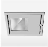
Recessed luminaire with LED, rated life of the LED L80/B10 > 50000 h, colour rendering index CRI > 96, chromaticity tolerance 2 SDCM (initial), reflector with asymmetrical light distribution pattern, reflector pure aluminium 99,99% in MIRO-Silver®, swivel angle 30°, luminaire housing sheet steel, powdercoated, stratosilver, separate driver unit
