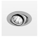
Recessed luminaire with LED, rated life of the LED L80/B10 > 50000 h, colour rendering index CRI > 90, chromaticity tolerance 2 SDCM (initial), rotation-symmetrical reflector with circular light distribution pattern, reflector pure aluminium 99,99% in MIRO-Silver®, segmented and faceted, 3D lens silicon to reduce the proportion of scattered light, die-cast aluminium, powder-coated, rotation angle, swivel angle +25° / -25°, stratosilver,
