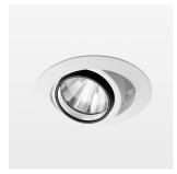
Recessed luminaire with LED, rated life of the LED L80/B10 > 50000 h, colour rendering index CRI > 96, chromaticity tolerance 2 SDCM (initial), rotation-symmetrical reflector with circular light distribution pattern, reflector pure aluminium 99,99% in MIRO-Silver®, segmented and faceted, 3D lens silicon to reduce the proportion of scattered light, die-cast aluminium, powder-coated, rotation angle, swivel angle +25°/-25°, stratowhite,
