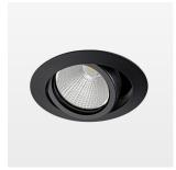
Recessed luminaire with LED, rated life of the LED L80/B10 > 50000 h, colour rendering index CRI > 96, chromaticity tolerance 2 SDCM (initial), reflector with circular light distribution pattern, reflector pure aluminium 99,99% in MIRO-Silver®, segmented and faceted, 3D lens silicon to reduce the proportion of scattered light, die-cast aluminium, powder-coated, rotation angle , swivel angle +25° / -25°, stratoblack,
