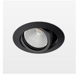
Recessed luminaire with LED, rated life of the LED L80/B10 > 50000 h, colour rendering index CRI > 96, chromaticity tolerance 2 SDCM (initial), reflector with circular light distribution pattern, reflector pure aluminium 99,99% in MIRO-Silver®, segmented and faceted, 3D lens silicon to reduce the proportion of scattered light, die-cast aluminium, powder-coated, rotation angle , swivel angle  $\pm 25^{\circ}$  /  $\pm 25^{\circ}$ , stratoblack,
