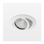
Recessed luminaire with LED, rated life of the LED L80/B10 > 50000 h, colour rendering index CRI > 80, chromaticity tolerance 2 SDCM (initial), reflector with circular light distribution pattern, reflector pure aluminium 99,99% in MIRO-Silver®, segmented and faceted, 3D lens silicon to reduce the proportion of scattered light, die-cast aluminium, powder-coated, rotation angle , swivel angle +25° / -25°, stratowhite,
