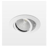
Recessed luminaire with LED, rated life of the LED L80/B10 > 50000 h, colour rendering index CRI > 96, chromaticity tolerance 2 SDCM (initial), reflector with circular light distribution pattern, reflector pure aluminium 99,99% in MIRO-Silver®, segmented and faceted, 3D lens silicon to reduce the proportion of scattered light, die-cast aluminium, powder-coated, rotation angle , swivel angle  $\pm 25^{\circ}$  /  $\pm 25^{\circ}$ , stratowhite,
