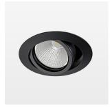
Recessed luminaire with LED, rated life of the LED L80/B10 > 50000 h, colour rendering index CRI > 90, chromaticity tolerance 2 SDCM (initial), reflector with circular light distribution pattern, reflector pure aluminium 99,99% in MIRO-Silver®, segmented and faceted, 3D lens silicon to reduce the proportion of scattered light, die-cast aluminium, powder-coated, rotation angle , swivel angle  $\pm 25^{\circ}$  /  $\pm 25^{\circ}$ , stratoblack,
