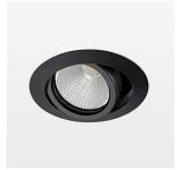
Recessed luminaire with LED, rated life of the LED L80/B10 > 50000 h, colour rendering index CRI > 80, chromaticity tolerance 2 SDCM (initial), reflector with circular light distribution pattern, reflector pure aluminium 99,99% in MIRO-Silver®, segmented and faceted, 3D lens silicon to reduce the proportion of scattered light, die-cast aluminium, powder-coated, rotation angle , swivel angle  $\pm 25^{\circ}$  /  $\pm 25^{\circ}$ , stratoblack,
