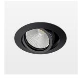
Recessed luminaire with LED, rated life of the LED L80/B10 > 50000 h, colour rendering index CRI > 90, chromaticity tolerance 2 SDCM (initial), reflector with circular light distribution pattern, reflector pure aluminium 99,99% in MIRO-Silver®, segmented and faceted, 3D lens silicon to reduce the proportion of scattered light, die-cast aluminium, powder-coated, rotation angle , swivel angle +25° / -25°, stratoblack,
