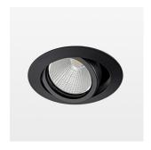
Recessed luminaire with LED, rated life of the LED L80/B10 > 50000 h, colour rendering index CRI > 96, chromaticity tolerance 2 SDCM (initial), reflector with circular light distribution pattern, reflector pure aluminium 99,99% in MIRO-Silver®, segmented and faceted, 3D lens silicon to reduce the proportion of scattered light, die-cast aluminium, powder-coated, rotation angle , swivel angle +25° / -25°, stratoblack,
