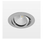
Recessed luminaire with LED, rated life of the LED L80/B10 > 50000 h, colour rendering index CRI > 96, chromaticity tolerance 2 SDCM (initial), reflector with circular light distribution pattern, reflector pure aluminium 99,99% in MIRO-Silver®, segmented and faceted, 3D lens silicon to reduce the proportion of scattered light, die-cast aluminium, powder-coated, rotation angle , swivel angle +25° / -25°, stratosilver,
