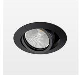
Recessed luminaire with LED, rated life of the LED L80/B10 > 50000 h, colour rendering index CRI > 80, chromaticity tolerance 2 SDCM (initial), reflector with circular light distribution pattern, reflector pure aluminium 99,99% in MIRO-Silver®, segmented and faceted, die-cast aluminium, powder-coated, rotation angle , swivel angle +25° / -25°, stratoblack,
