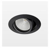
Recessed luminaire with LED, rated life of the LED L80/B10 > 50000 h, colour rendering index CRI > 96, chromaticity tolerance 2 SDCM (initial), reflector with circular light distribution pattern, reflector pure aluminium 99,99% in MIRO-Silver®, segmented and faceted, die-cast aluminium, powder-coated, rotation angle , swivel angle +25° / -25°, stratoblack,
