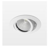
Recessed luminaire with LED, rated life of the LED L80/B10 > 50000 h, colour rendering index CRI > 90, chromaticity tolerance 2 SDCM (initial), reflector with circular light distribution pattern, reflector pure aluminium 99,99% in MIRO-Silver®, segmented and faceted, die-cast aluminium, powder-coated, rotation angle, swivel angle +25° / -25°, stratowhite,
