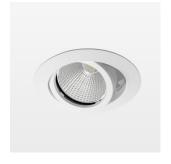
Recessed luminaire with LED, rated life of the LED L80/B10 > 50000 h, colour rendering index CRI > 80, chromaticity tolerance 2 SDCM (initial), reflector with circular light distribution pattern, reflector pure aluminium 99,99% in MIRO-Silver®, segmented and faceted, die-cast aluminium, powder-coated, rotation angle , swivel angle +25° / -25°, stratowhite,
