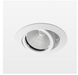
Recessed luminaire with LED, rated life of the LED L80/B10 > 50000 h, colour rendering index CRI > 96, chromaticity tolerance 2 SDCM (initial), reflector with circular light distribution pattern, reflector pure aluminium 99,99% in MIRO-Silver®, segmented and faceted, die-cast aluminium, powder-coated, rotation angle , swivel angle +25° / -25°, stratowhite,
