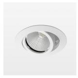
Recessed luminaire with LED, rated life of the LED L80/B10 > 50000 h, colour rendering index CRI > 96, chromaticity tolerance 2 SDCM (initial), reflector with circular light distribution pattern, reflector pure aluminium 99,99% in MIRO-Silver®, segmented and faceted, die-cast aluminium, powder-coated, rotation angle , swivel angle +25° / -25°, stratowhite,
