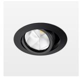
Recessed luminaire with LED, rated life of the LED L80/B10 > 50000 h, colour rendering index CRI > 90, chromaticity tolerance 2 SDCM (initial), reflector with oval light distribution pattern, reflector pure aluminium 99,99% in MIRO-Silver®, segmented, die-cast aluminium, powder-coated, rotation angle , swivel angle  $\pm 25^{\circ}$  /  $\pm 25^{\circ}$ , stratoblack,
