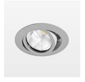
Recessed luminaire with LED, rated life of the LED L80/B10 > 50000 h, colour rendering index CRI > 96, chromaticity tolerance 2 SDCM (initial), reflector with oval light distribution pattern, reflector pure aluminium 99,99% in MIRO-Silver®, segmented, die-cast aluminium, powder-coated, rotation angle , swivel angle  $+25^{\circ}$  /  $-25^{\circ}$ , stratosilver,
