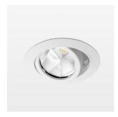
Recessed luminaire with LED, rated life of the LED L80/B10 > 50000 h, colour rendering index CRI > 96, chromaticity tolerance 2 SDCM (initial), reflector with oval light distribution pattern, reflector pure aluminium 99,99% in MIRO-Silver®, segmented, die-cast aluminium, powder-coated, rotation angle , swivel angle  $\pm 25^{\circ}$  /  $\pm 25^{\circ}$ , stratowhite,
