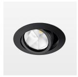
Recessed luminaire with LED, rated life of the LED L80/B10 > 50000 h, colour rendering index CRI > 96, chromaticity tolerance 2 SDCM (initial), reflector with oval light distribution pattern, reflector pure aluminium 99,99% in MIRO-Silver®, segmented, die-cast aluminium, powder-coated, rotation angle , swivel angle  $\pm 25^{\circ}$  /  $\pm 25^{\circ}$ , stratoblack,
