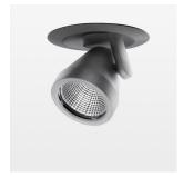
Semi-recessed luminaire with LED, rated life of the LED L80/B10 > 50000 h, colour rendering index CRI > 90, chromaticity tolerance 2 SDCM (initial), rotation-symmetrical reflector with circular light distribution pattern, reflector pure aluminium 99,99% in MIRO-Silver®, segmented and faceted, 3D lens silicon to reduce the proportion of scattered light, die-cast aluminium, powder-coated, rotation angle 400°, swivel angle +85° / -85°, stratosilver, separate driver unit
