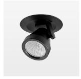
Semi-recessed luminaire with LED, rated life of the LED L80/B10 > 50000 h, colour rendering index CRI > 80, chromaticity tolerance 2 SDCM (initial), reflector with circular light distribution pattern, reflector pure aluminium 99,99% in MIRO-Silver®, segmented and faceted, 3D lens silicon to reduce the proportion of scattered light, die-cast aluminium, powder-coated, rotation angle 400°, swivel angle +85° / -85°, stratoblack, separate driver unit
