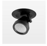
Semi-recessed luminaire with LED, rated life of the LED L80/B10 > 50000 h, colour rendering index CRI > 80, chromaticity tolerance 2 SDCM (initial), reflector with circular light distribution pattern, reflector pure aluminium 99,99% in MIRO-Silver®, segmented and faceted, 3D lens silicon to reduce the proportion of scattered light, die-cast aluminium, powder-coated, rotation angle 400°, swivel angle +85° / -85°, stratoblack, separate driver unit
